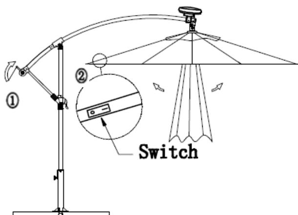
7. ① Wind the crank handle to open the canopy.
