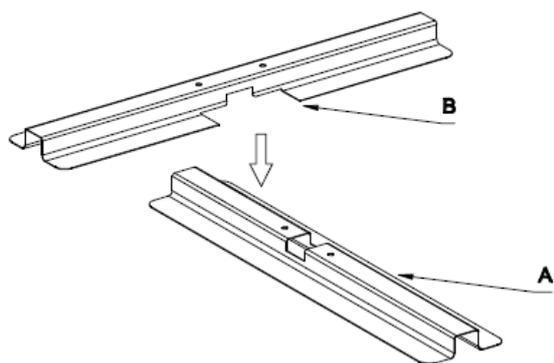
1. Join the base by placing B perpendicular on top of A.
