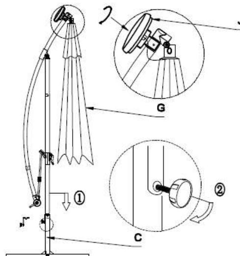
4. Attach the solar panel (J) by connecting the wire at the top of the parasol and twisting into the holder.
