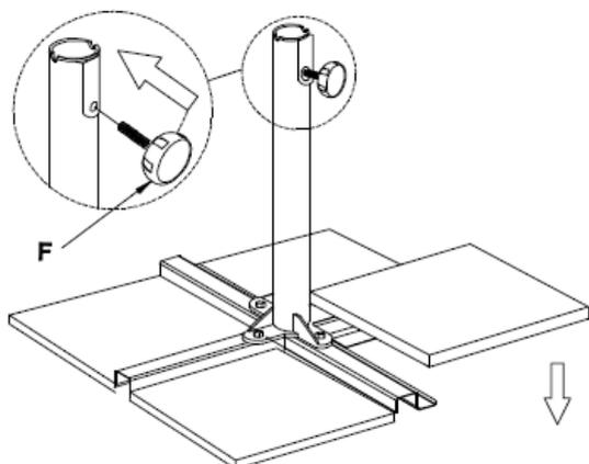
3. Loosely attach the securing bolt (F) as shown.
